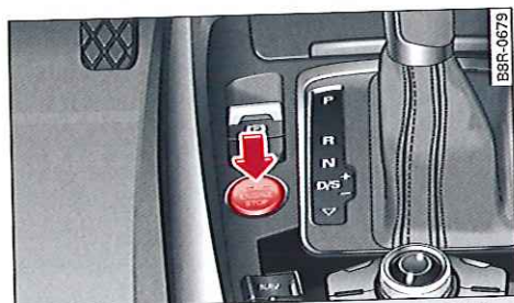
Fig. 101 Console centrale : touche START ENGINE STOP
