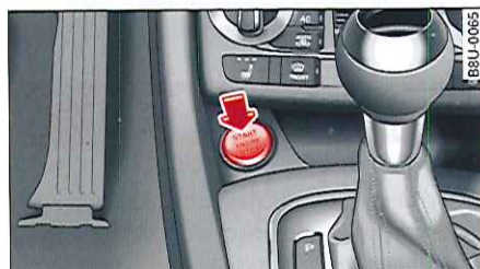
Fig. 82 Console centrale : touche START ENGINE STOP
