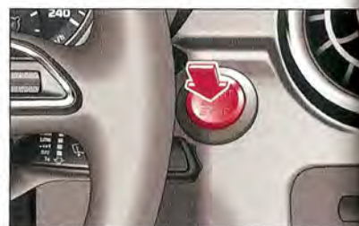
Fig. 80 Console centrale : touche START ENGINE STOP (clé confort)
